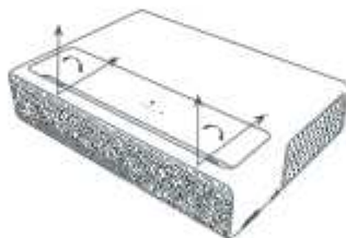
Front sensor range: Approximately 55°
