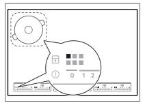
Each square on the control panel represents one cooking zone on the induction cooking surface. Zone indicators show which cooking zone is controlled by the appropriate control bar.
