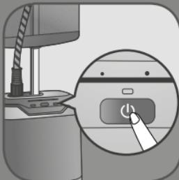
**EN** The appliance must be switched off, push the ON/OFF button in order to switch it off.
