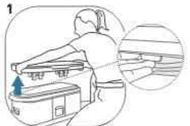
1-Raise the shutter slightly to across the handles. Press in the shutter lock/handle, then remove the top cover from the base.
