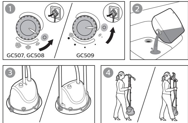
**EN** Always empty the water tank after usage, to prevent calc build-up and maintain good steam performance.
