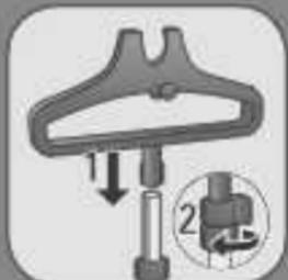
**EN** Unlock the hanger and fully insert it vertically on top of the pole and lock it.
