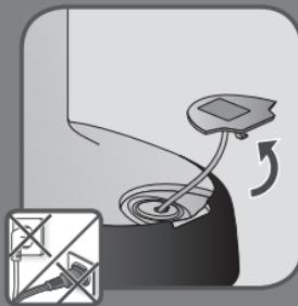
**EN** Open the water inlet cap and fill the beaker with water up to the maximum limit.
