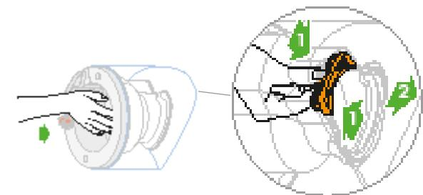
To attach the loop amplifier surround, lie flat and align the surround to the main amplifier. Push firmly until it clicks into place as shown.
