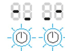
Water treatment: The AM10 is treating the water. This takes 3 minutes. When the animation stops, the AM10 will start to humidify.
