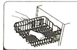
1 To raise the upper basket, just lift the upper basket at the center of each side until the basket locks into place in the upper position. It is not necessary to lift the adjuster handle.
