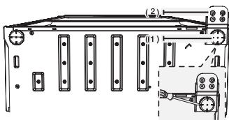
8. Replace the position of the lower leg and bracket (right-to left)
