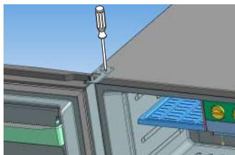
16. Insert the top gasket into the holder and close the cover with a screw (+), a screwdriver.
