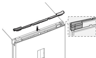
16. Change the direction of the cable door in the opposite direction and wipe the door cover.
