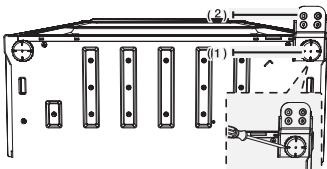
7. Carefully pack the refrigerator. Remove the roller (1) and foot (2)
