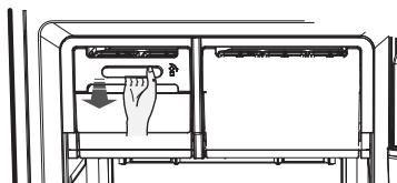
Be careful when removing the base of the ice cap, as it may suddenly shift towards you. On the pallets, hold the ice plate lever to the right, so be on the right. Holding the middle part down, slide the base of the ice cabin back into place.
