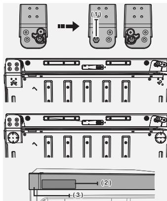
10. Change the posterior stem and foot (from left → to right). After installing the freezer door on the middle trim, wrap the bottom trim.
