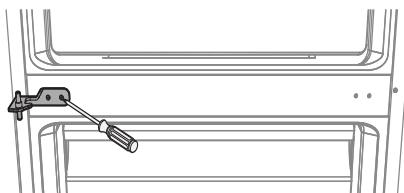
12. Using a 10 mm diameter probe, remove the grille.
