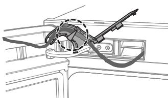
14. Connect the cord and place the control cable on the clamp cover, and then slide the knob to secure the connection, as shown in the following figure.
