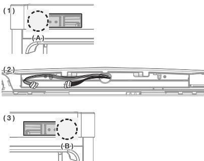
11. After removing the control panel cover (1), replace the direction of the door of the wires (2) in the direction opposite to the refrigerator door (only for the display model). Use screw (A) as shown in figure (3).
