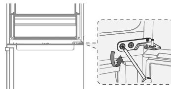
6. Carefully freeze the bottom of the freezer door to lift it up. The door is open, so be careful not to get hurt when removing the door.
