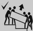
The refrigerator must be raised by two or three people and must be sure that the surface is installed vertically.
