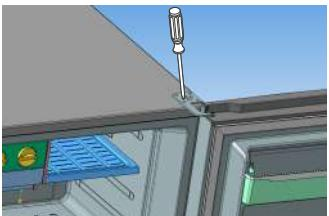
3. Remove the blind door vertically upwards by pulling it out of the center pillar.
