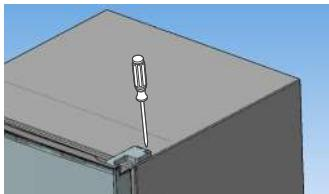
2. Then screw in the 3 screws of the upper tower using a transverse (+) conveyor and remove the upper rack.
