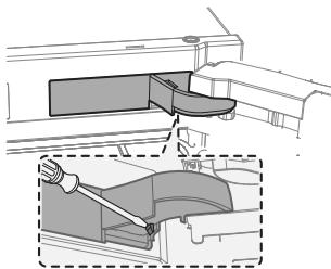
3. Disconnect the wires (for doors with a screen display). Then attach the top screw to the screw with two screws and remove the strap.
