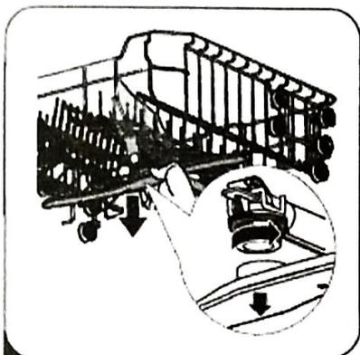
**1** To remove the upper spray arm, hold the nut in the center still and rotate the spray arm counterclockwise to remove it.
