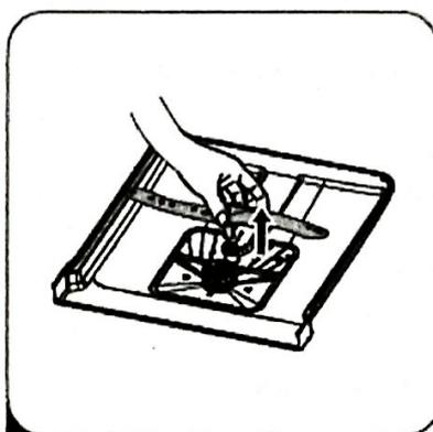
**2** To remove the lower spray arm, pull out the spray arm upward.
