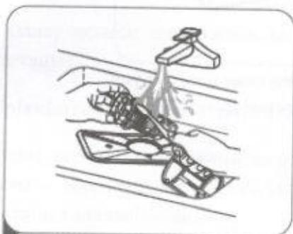
**3** Larger food remnants can be cleaned by rinsing the filter under running water. For a more thorough clean, use a soft cleaning brush.
