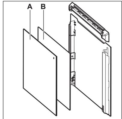
Make sure that you install the middle panel of glass in the seats correctly.
