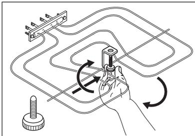
2. Carefully pull the heating element down.
