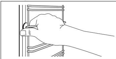
2. Pull the rear end of the shelf support away from the side wall and remove it.
