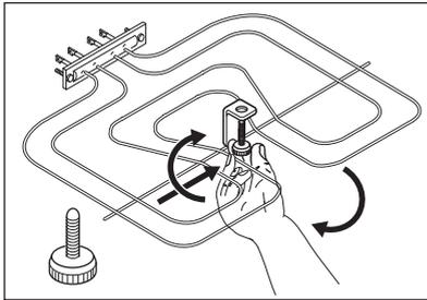
2. Carefully pull the heating element down.
