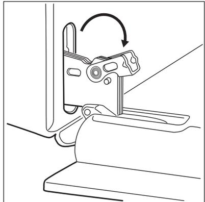
5. Close the oven door halfway to the first opening position. Then lift and pull forward and remove the door from its seat.
