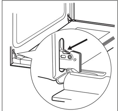
4. Lift and turn the lever fully on the left hinge.
