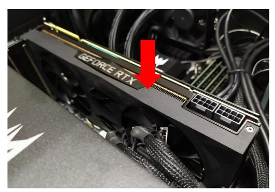
4. Secure the Graphic board with screws.
