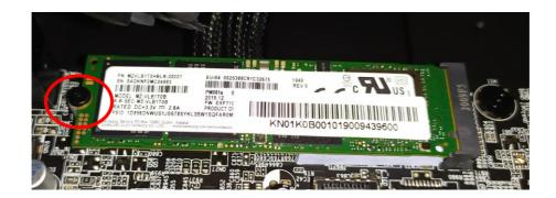
4. Detach the M.2 SSD module from the mainboard.
