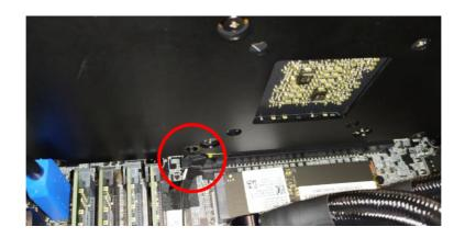
5. Detach the Graphic board from the PCIe x16 slot.
