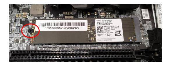
4. Detach the M.2 SSD module from the mainboard.
