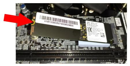
3. Secure the M.2 SSD module and mainboard with screws.
