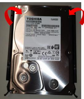
3. Insert black rack into HDD cage.
