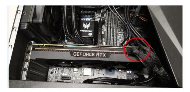
3. Remove the screw that secure the Graphic boards to the chassis.
