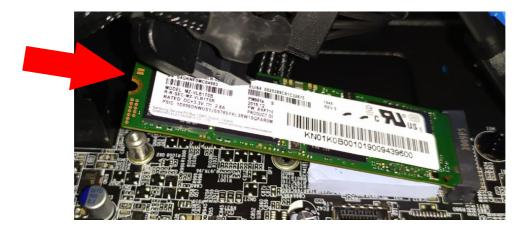
3. Secure the M.2 SSD module and mainboard with screws.
