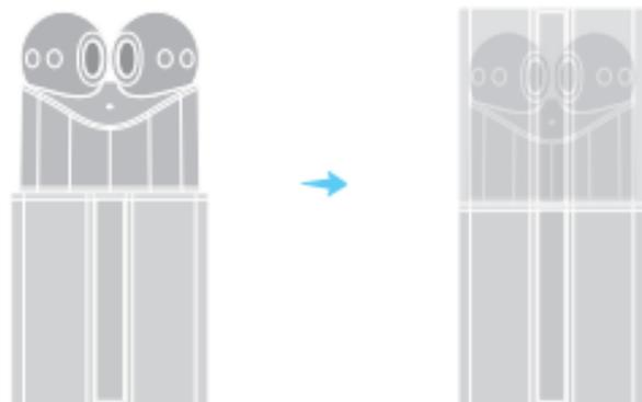
**EN** Place the earphones in the charging case and close the case. They will start charging automatically.
