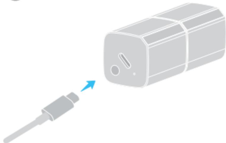
**EN** Connect the case to a USB-C cable to charge it.
