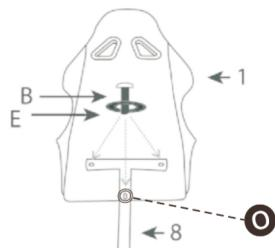
**6. Insert the backrest mount into the hole in the butterfly mechanism and secure it by turning the handle.**
