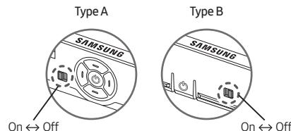
You can turn on or off the microphone by using the switch at the bottom of the TV. If microphone is turned off, All voice and sound features using microphone are not available.
