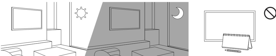
Eco Sensor adjusts the brightness of the TV automatically. This feature measures the light in your room and optimises the brightness of the TV automatically to reduce power consumption. If you want to turn this off, go to > Settings > General > Eco Solution > Ambient Light Detection.
